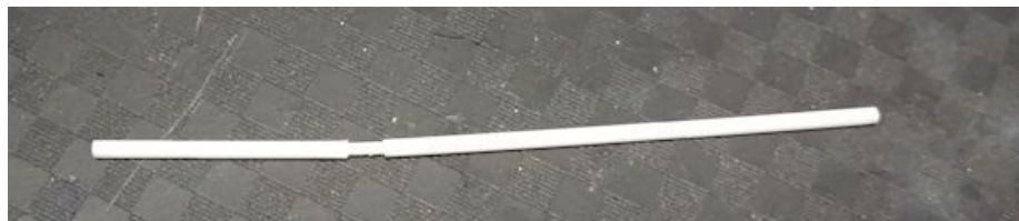
Figure 3.9: Strut inserted into both pieces of tube before glue is applied and they can be pushed together.
